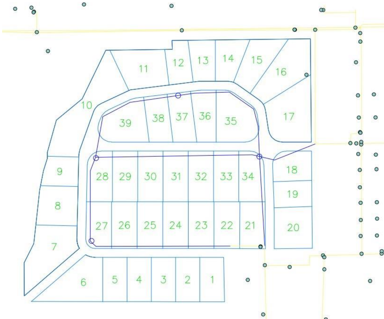
Figure 17: Final Water Main Design with Existing Utilities
