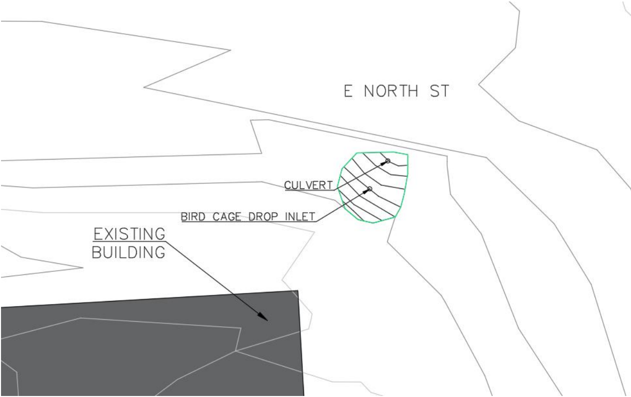
Figure B.1: Proposed drain surface
