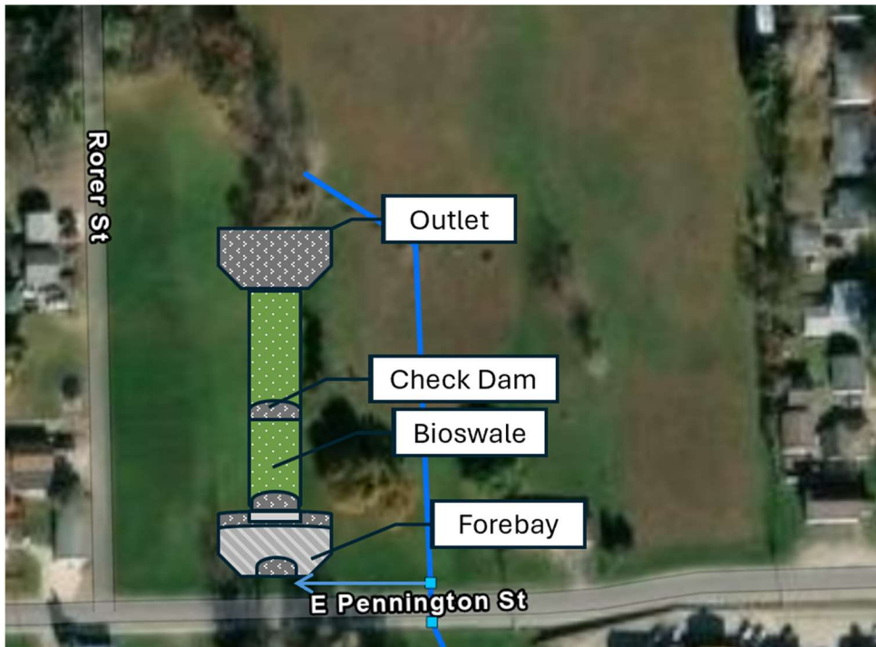
Figure 9: Approximate size and location of the proposed bioswale.
