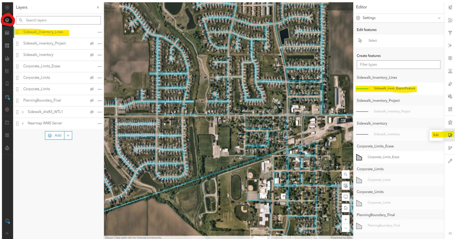
Figure 1: Interface of sidewalks Web Map. Clicking the highlighted “Sidewalk_inven_ExportFeature” allows the users to add lines over new sidewalks.
