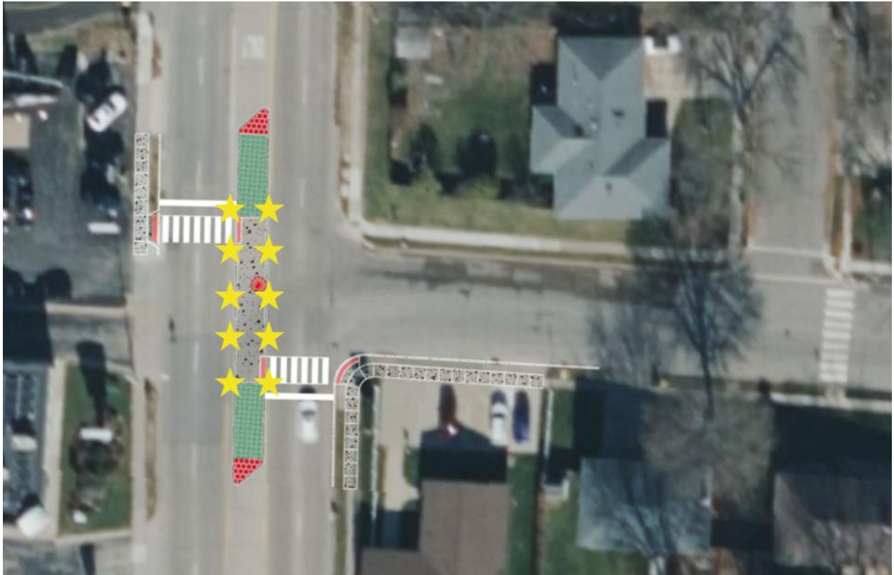
Figure 35. Ideal placement of the flexible delineators on the pedestrian median as denoted by a star.
