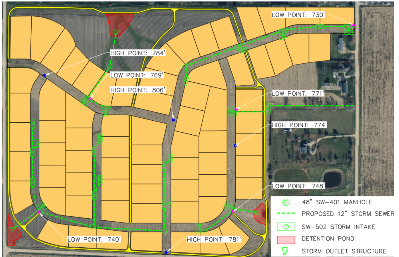
Figure 20: Proposed Storm Sewer
