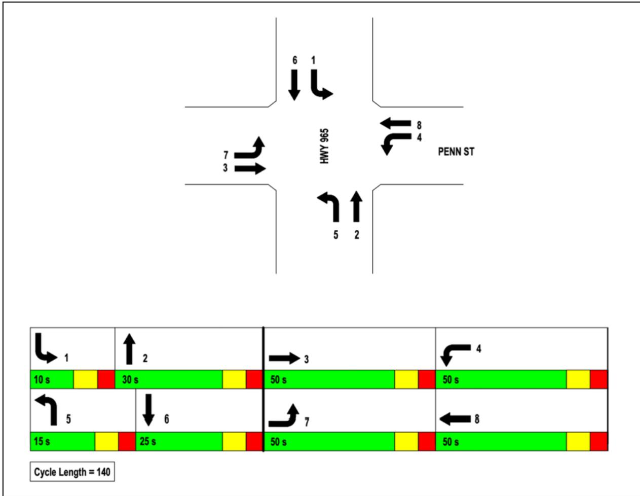
Figure 11: Phasing and Timing Plan.
