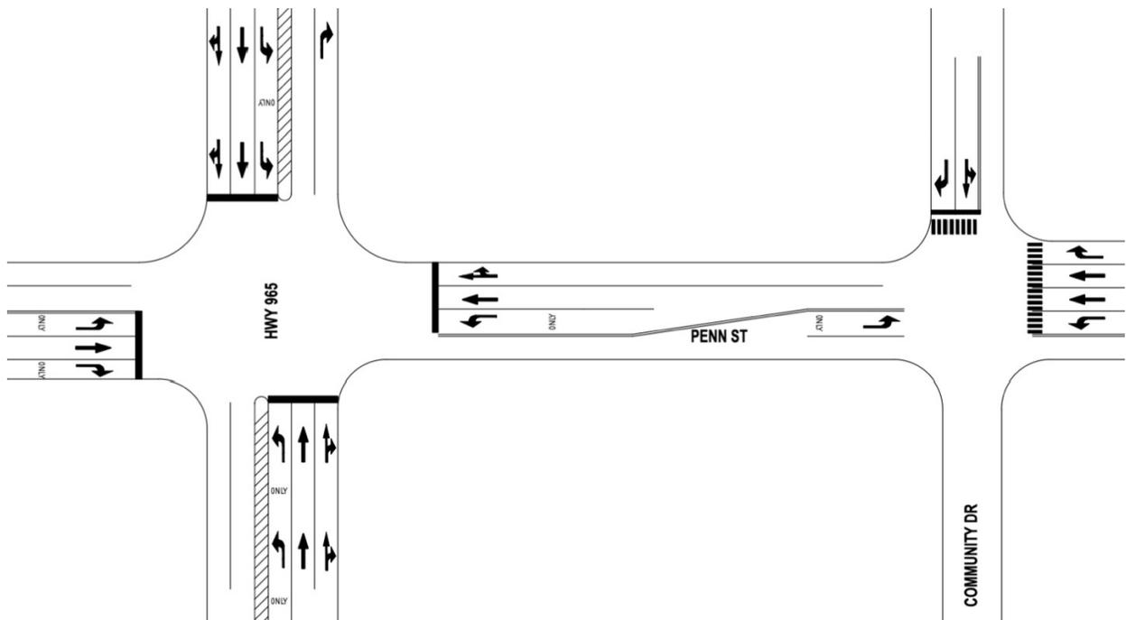
*Figure 13: Widening the right of way alternative illustration.*
