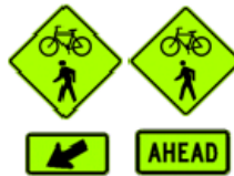
Figure 12: Required dot pedestrian crossing signage.
