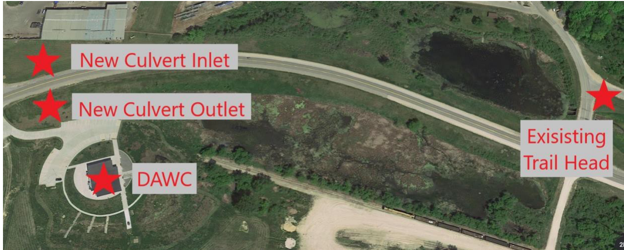
Figure 5: Proposed new culvert location.
