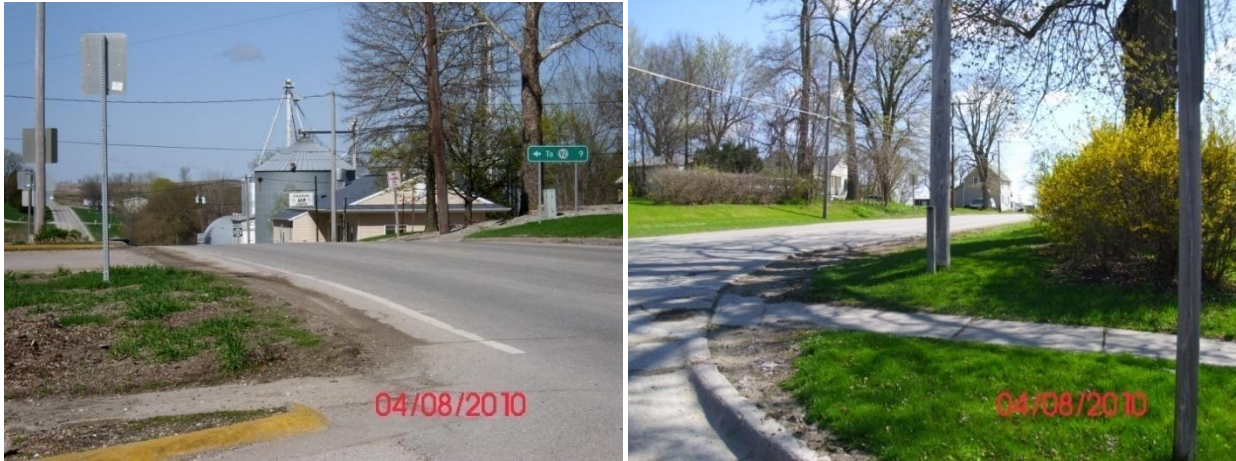
Limited site-distance and visibility at 8 th (left) and 7 th (right) avenues make pedestrian crossing difficult and potentially unsafe. Traffic control devices such as stop or yield signs or speed bumps would help encourage lower speeds along this corridor and make crossing less hazardous. Photos: Sheila Knoploh-Odole
