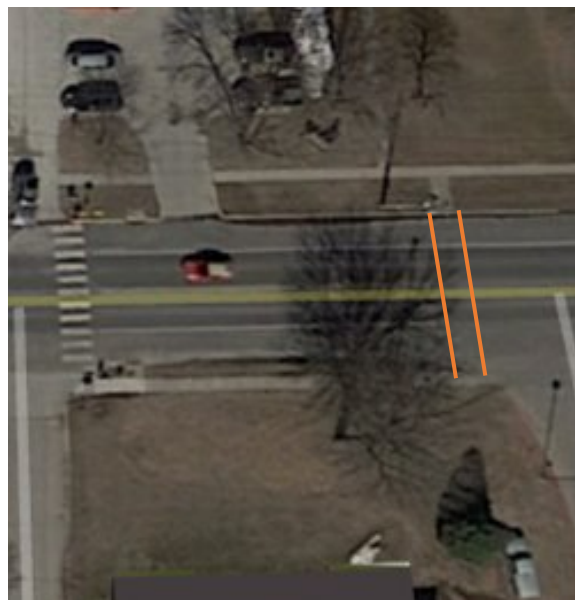
Figure 8. Proposed location for the relocation of the pedestrian crossing.
