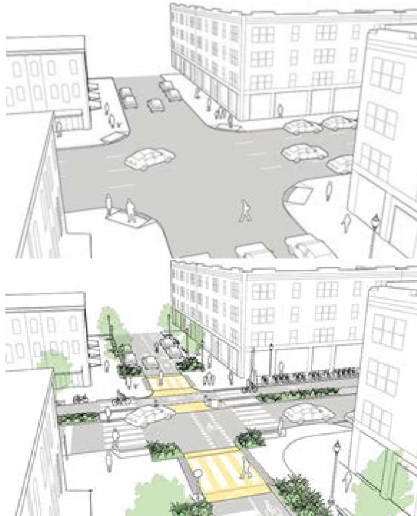
Figure 37: Example of intersections improvements
