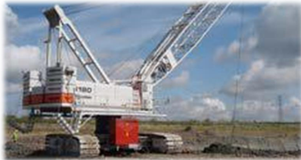
A crawler crane. Source: Norman Spencer
