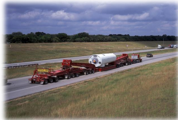
A 19-axle trailer carrying a nacelle. Source: TrailKing Industries
