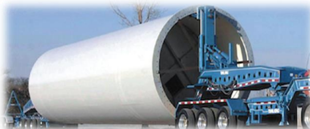
A Schnabel trailer holding a wind turbine tower section. Source: WindPower Engineering
