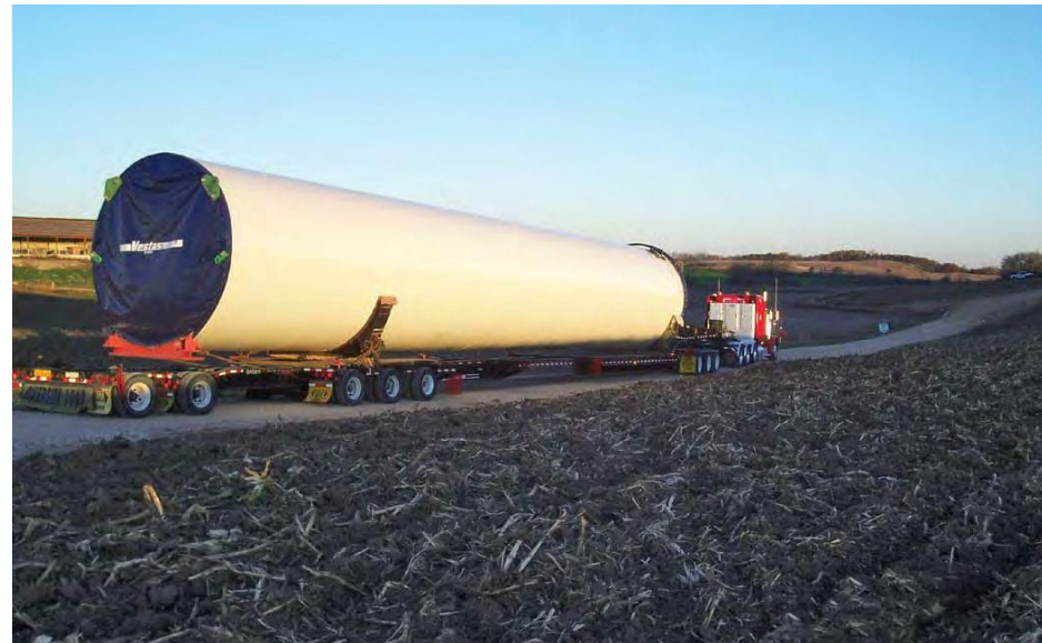
Transporting a wind turbine tower section to the construction site. Source: (WE Energies 2012)
