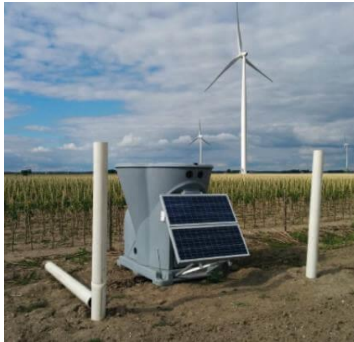
A picture of the Triton SoDAR device at the Ecofys Testing Site in Lelystad, Netherlands. Source: (Dvorak 2016)
