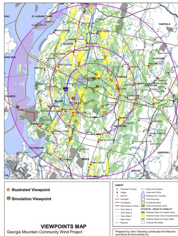
Figure 47: An example of a viewshed analysis map with selected viewpoints Adapted from Vissering, Sinclair, and Morgolis, 20111
