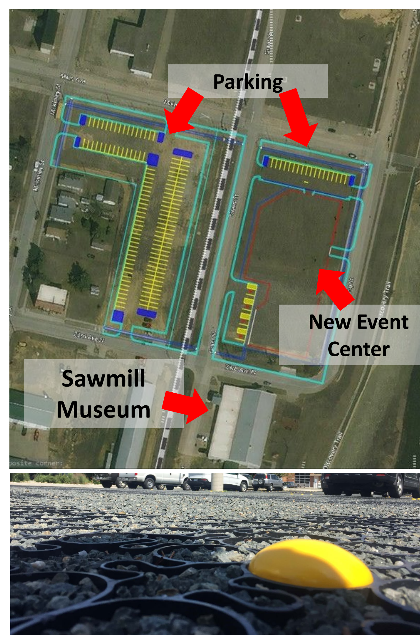
Figure 2. Site layout and True Grid™ pavers
