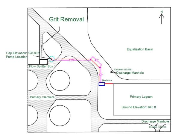
Figure 6: The piping network design option 1 layout. The pipes are shown in red, the light blue circle indicate the starting point and pump location, and the magenta lines are length measurements. The headerbox is the royal blue rectangle.
