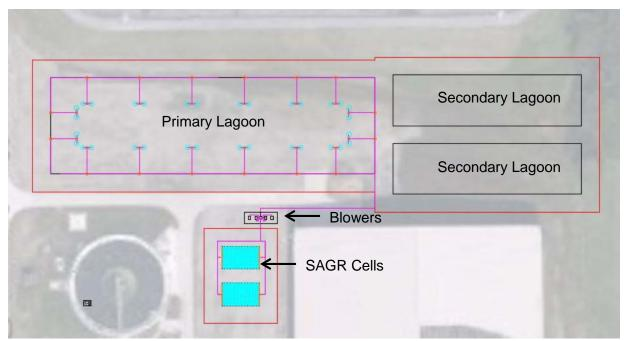
Figure 11: Overall Blower System Layout
