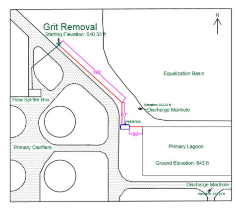
Figure 9: The piping network design option 4 layout. The pipes are shown in red, the blue circles indicate the starting points, and the magenta lines are length measurements. The headerbox is the royal blue rectangle.
