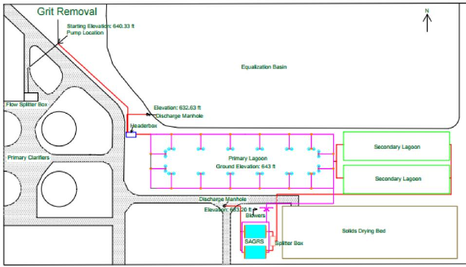
Figure 14: Final Pipe and Lagoon Design
