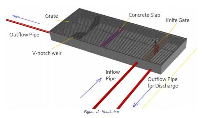
The water first enters a space that will allow the flow to calm. On the west side, there will be a wall with a 6-inch diameter knife gate that will allow the excess flow to be routed to the start of the WWTP. The overflow line will start at the northwest corner of the headerbox at an elevation of 643.5 feet and travel north, then bend 90-degrees and run east until it reaches a manhole for the waste line that runs through the WWTP to the head of the plant. An image of the
