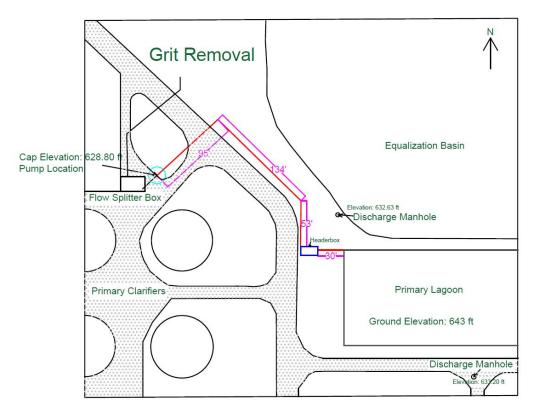
Figure 7: The piping network design option 2 layout. The pipes are shown in red, the blue circles indicate the starting point and pump location, and the magenta lines are length measurements. The headerbox is the royal blue rectangle.
