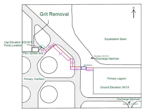
Figure 8: The piping network design option 3 layout. The pipes are shown in red, the blue circles indicate the starting point and pump location, and the magenta lines are length measurements. The headerbox is the royal blue rectangle.
