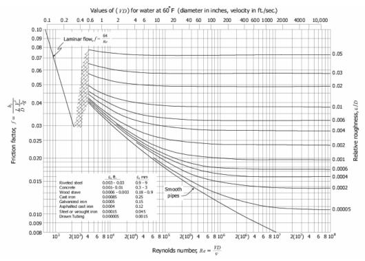
Figure 15: Moody diagram used to determine f by following the smooth pipes curve for different Re values.
