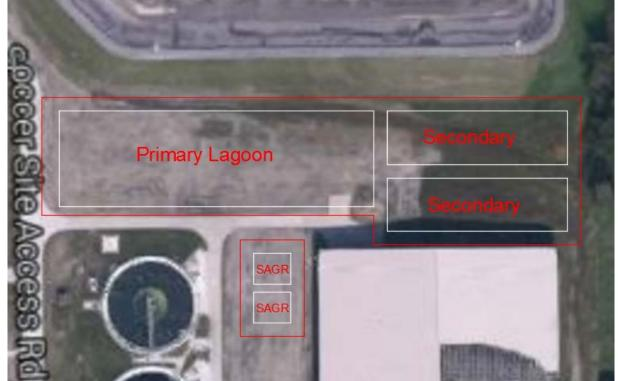
Figure 5: Final Design Layout of Lagoon and SAGR System
