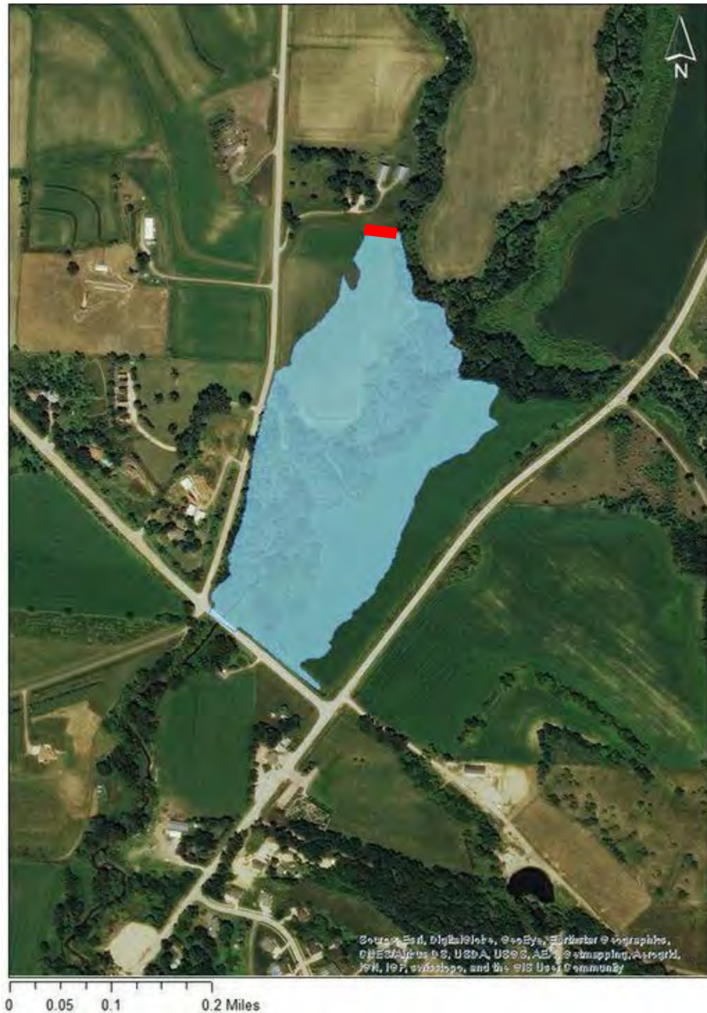
Figure 5: Aerial view of dry detention basin with berm (red) at S. Ridge Rd.
