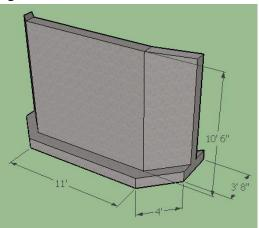
Figure 9: 3D rendering of pedestrian bridge abutment
