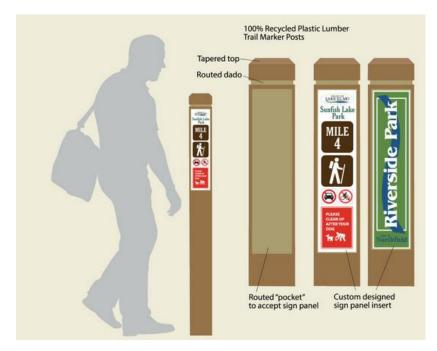
Figure 10: Recycled plastic lumber mile marker posts, courtesy of Vacker Signs Inc.
