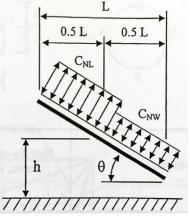
Figure A1: Roof wind loading
