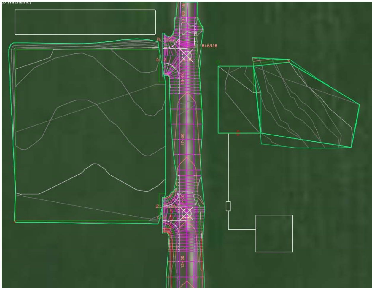
Figure 2: A close aerial view of the site work from station 15-00 to station 19-00 of the new asphalt road
