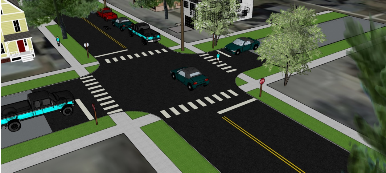
Figure B4. Rendering showing new four-way stop control at the 2 nd St. SE intersection
