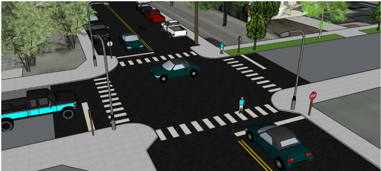
Figure 15. E. State St. Intersection from Alternative One with existing crossing and lane widths. The pedestrian crossing distance across Pennsylvania Avenue is in excess of 45 feet.
