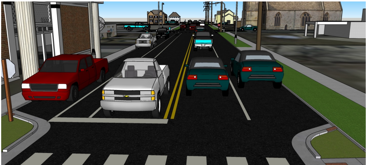
Figure 22. Rendering showing driver's viewpoint of wide bike lane with permitted parking during designated times.
