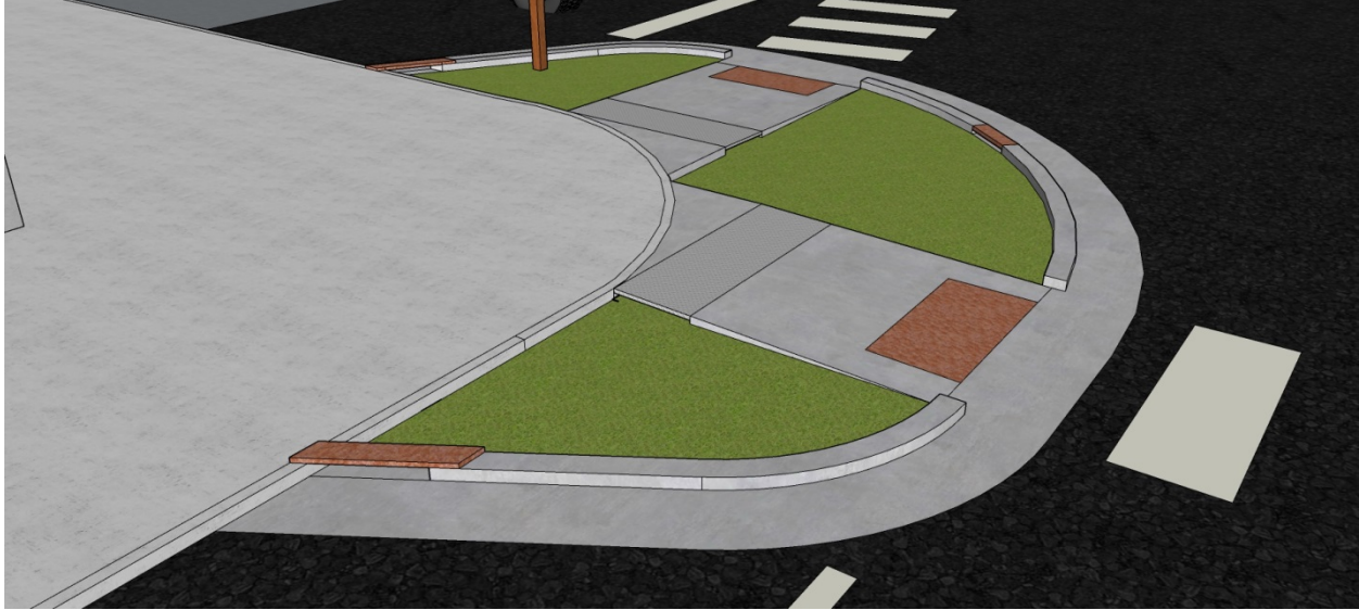
Figure C6. Side view of a typical bump-out showing relative elevations to the existing sidewalk and street.
