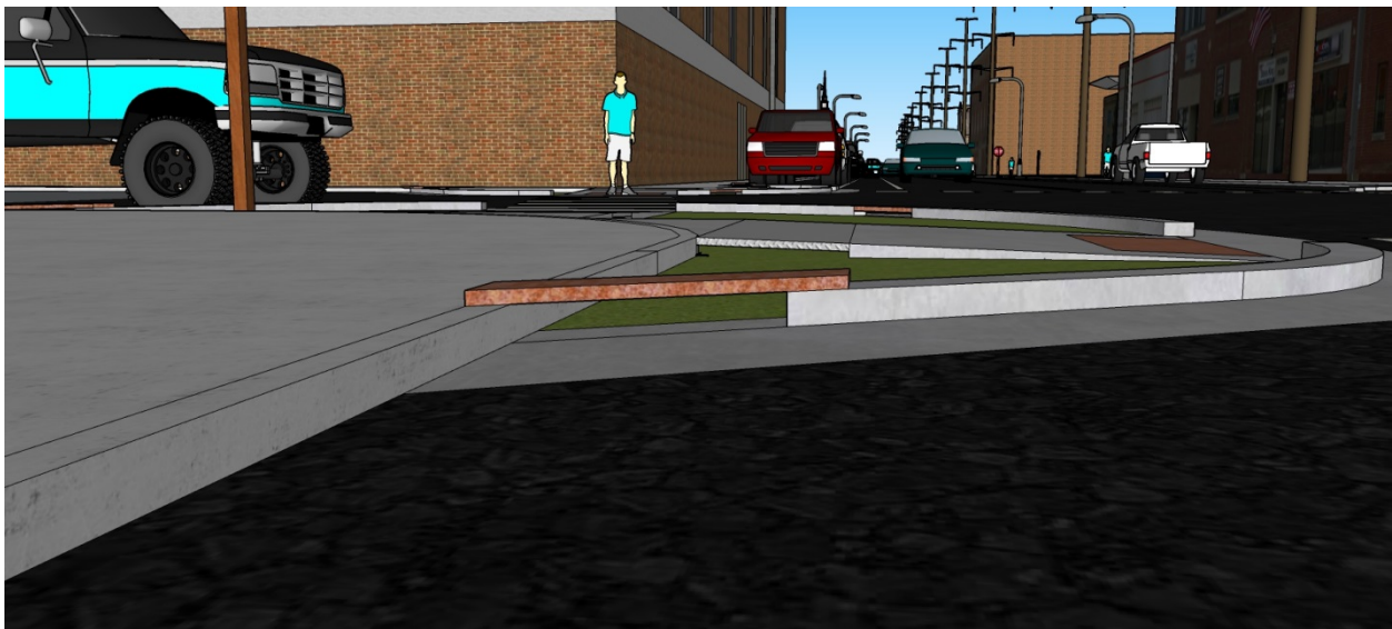
Figure C7. Rendering of steel plate over curb cut, which allows water to flow into the bump-out but keeps vehicles and bicycles from entering.
