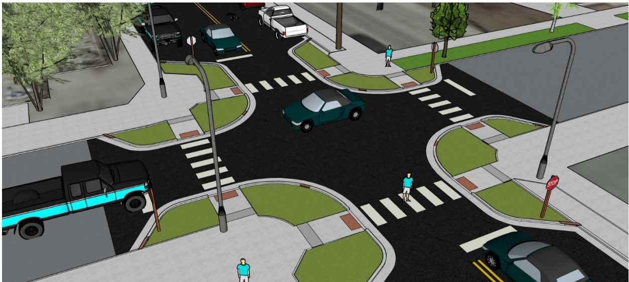
Figure 16. E. State St. Intersection in Alternative Two. Notice the reduced pedestrian crossing distances and reduced lane widths throughout the intersection. All pedestrian crossing distances have been reduced to 22 feet.
