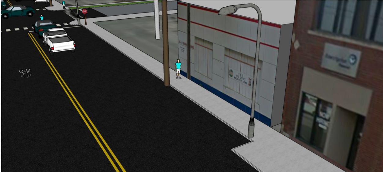
Figure 17. Curb not filled in along Pennsylvania Avenue, showing the potential hazard of the utility poles in the parking lane.
