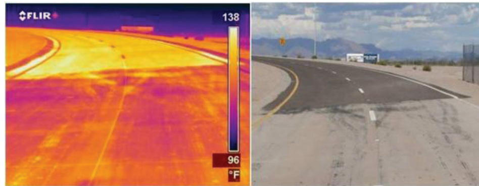
Figure 8. Temperature change in different colored pavements. Source: Heat Island Group.
