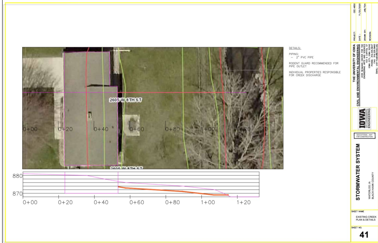
Figure 5: Plan and Profile for discharging to nearby creek
