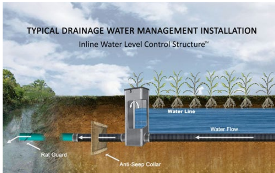
Figure 5.4. Typical drainage water management side profile
