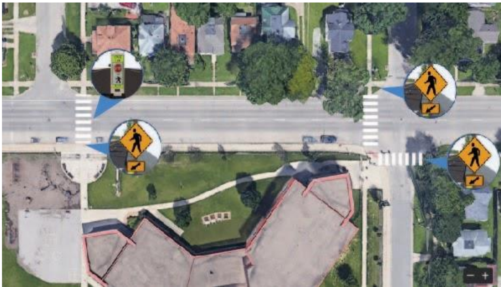
Figure 16: Example of high visibility crosswalk placement on 5th Street near Irvine Elementary
