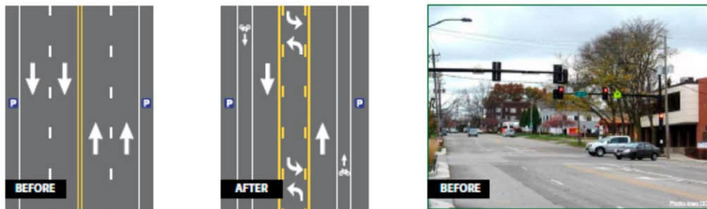
Figure 19: Des Moines' Ingersoll Avenue Road diet
