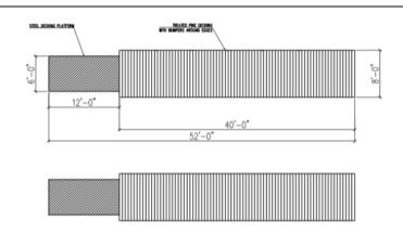
TYPICAL RETRACTABLE FLOATING BOAT DOCK DETAIL
