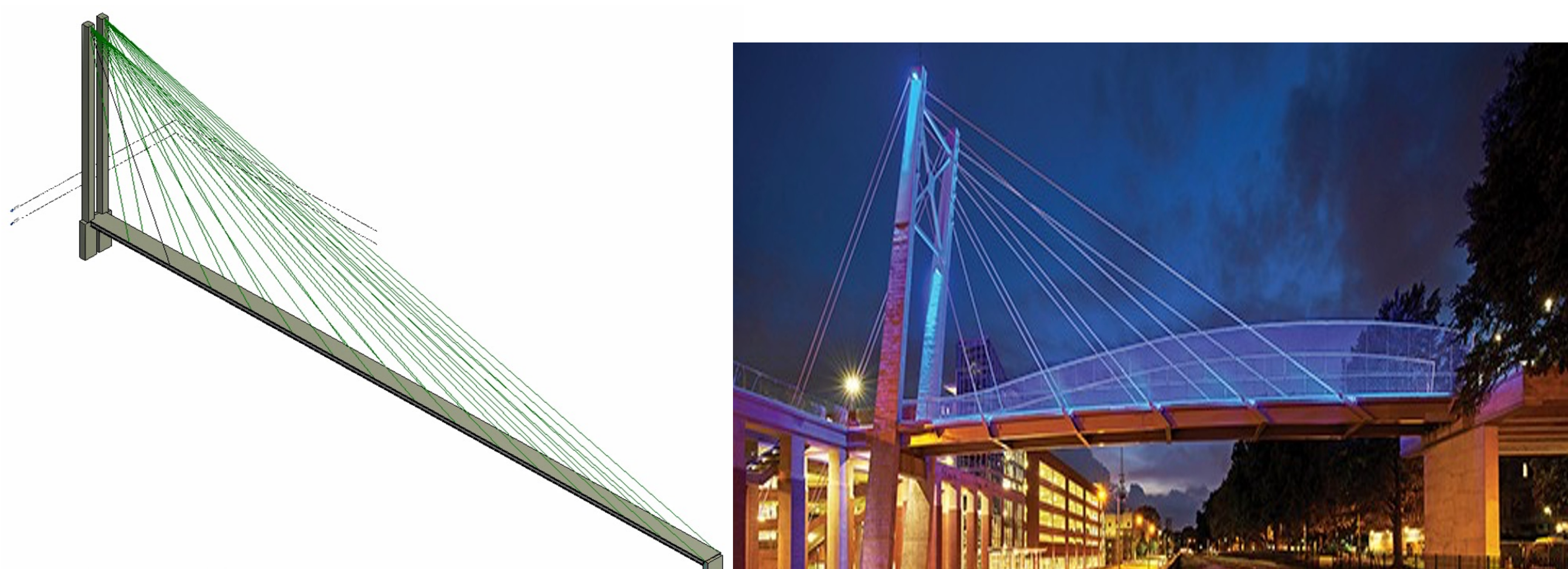
Figure 3 (left). A Revit model of the proposed bridge's superstructure. Figure 4 (right). Cable-stayed pedestrian bridge in Memphis , TN.
