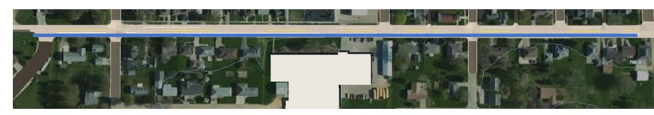
In order to improve connectivity between Easton Valley School and St. Joseph Church a pedestrian lane was designed to connect between Main St. and the church. The lane is 9 ft wide with a 2 ft painted buffer. Design was completed in accordance with the Small Town and Rural Design Guide for visually separated pedestrian lanes.
