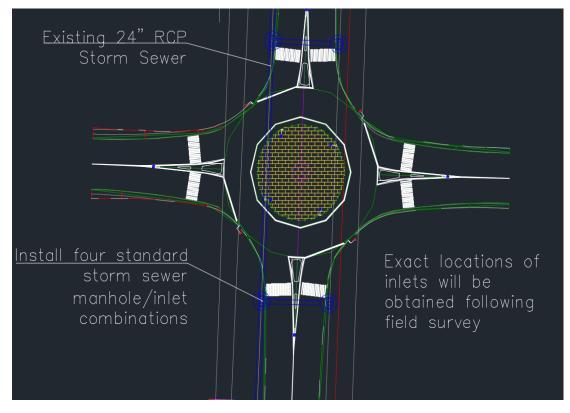
FIGURE 9: ROUNDABOUT STORM SEWER INLET CONSTRUCTION PLAN
