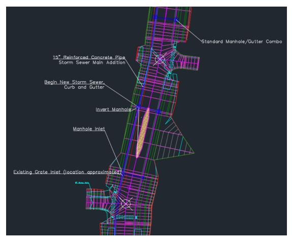
FIGURE 8: SAMPLE STORM SEWER EXTENSION PLAN
