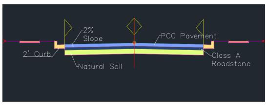
FIGURE 6: PAVEMENT DESIGN CROSS-SECTION
