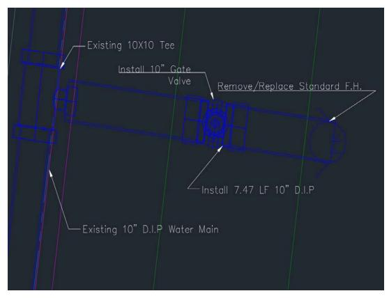
FIGURE 7: STATION 51+42.89 FIRE HYDRANT RELOCATION PLAN
