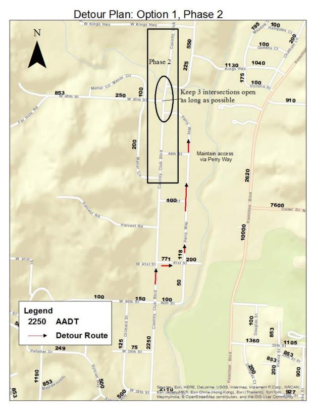
FIGURE 10B: PHASE TWO OF DETOUR PLAN, OPTION 1
