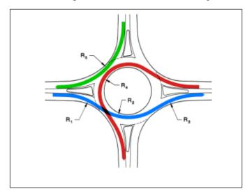
FIGURE 4: FIVE CRITICAL PATH RADII CRITERIA. SOURCE: FHWA ROUNDABOUT GUIDE EXHIBIT 6-12
