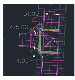
FIGURE 1A: INTERSECTION DETAIL WITH BRICK CROSSWALK
