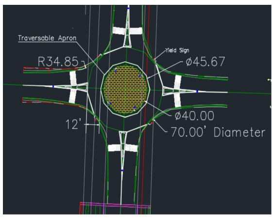
FIGURE 5: ROUNDABOUT DESIGN
